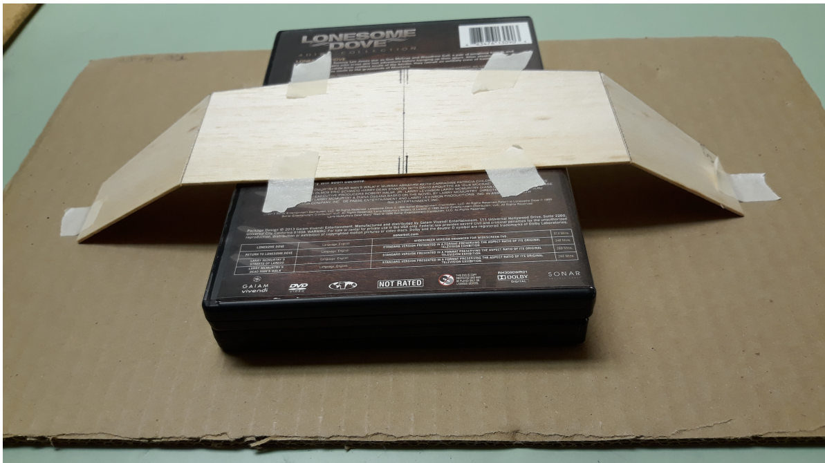
Wing tip dihedral joints. Wing is taped to DVD spacer and building board, prior to doubler installation.
