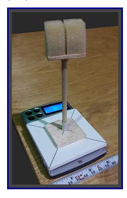
Gary Hodson's stand uses a plastic tube to hold the dowel. If you go this route and find your mast is a bit too loose, wrap Scotch tape around the base of the dowel or pencil to lessen the gap for a tighter fit.
